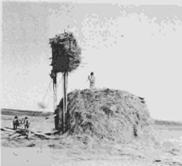
Over shot hay stacker that lifted hay from ground to hay stack.
